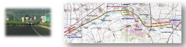
Section 45.1.4 (from Kostarazi to Argos Orestiko Interchange). The section, is located in the vertical axe towards Albania, in an high relief landscape with sequencing trenches and embankments. The section also contains a bridge of 420m of length and four complex interchanges.
