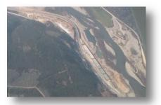
Section 1.1.4 (River Arahthos area). The project aimed on riverbed adjustment, under the new bridge (of length of 1.080m) serving Egnatia Highway. The river flood flux design estimation is of 800m<sup>3</sup>/sec.
